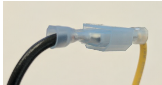
Figure 2 – Proper connection (male stab seated within female connector)
